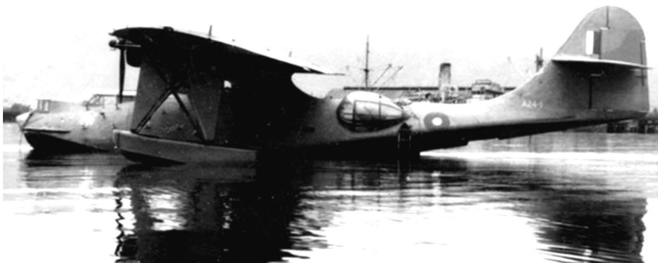
A24-1 of 11SQN at Cairns, probably in early 1943. TSS scheme, with a 2:5 proportioned 30" diameter roundel, dating this as 1943. Fin flash is 24" high and 16" wide (8" per colour). Nose art features Snifter .
