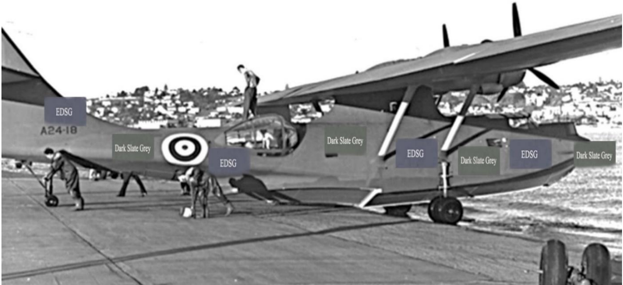
A24-18 on beaching gear in San Diego OCT 1941 with the TSS camouflage demarcation visible
