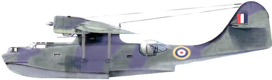
A faded 28-5MA delivery scheme – TSS RAF 35" type-A1 fuselage roundels, 72" type-B upper roundels, fin flash 24" x 24" 30 Dark Slate Grey had a marked greenish hue, EDSG faded quickly in the tropics to a bluish hue
