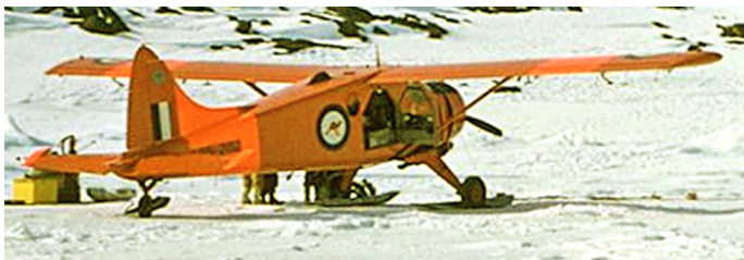
A95-202 with International Orange (FS12197) dayglo band around the rear fuselage and bands across the mainplanes – the image at right shows severe fading of the dayglo (added at Mawson during 1958).
