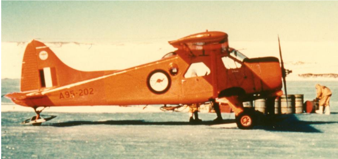
A95-202 139 showing dayglo bands on rear fuselage/fin and over and below the mainplanes – apparently added at Mawson in 1958, becoming the first RAAF aircraft with dayglo.
