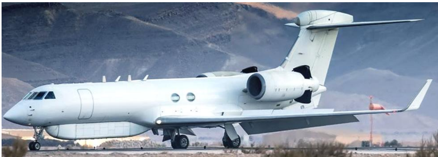
The RAAF AISREW variant – MC-55A – would look more like this, no conformal AEW radar and a ventral gondola
