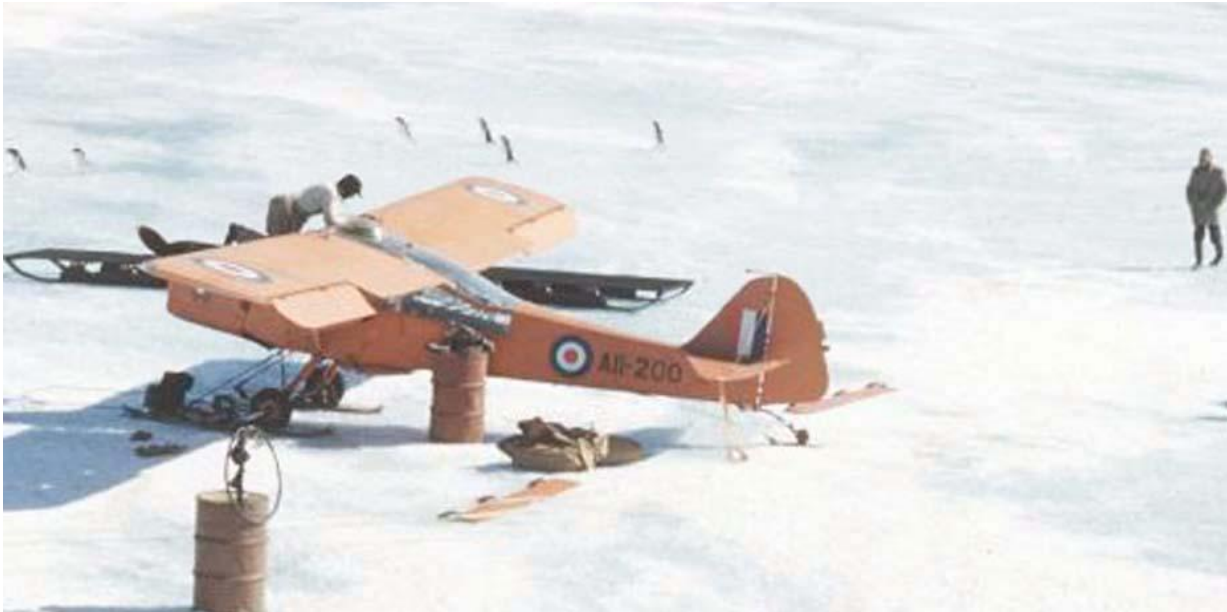
A11-200 on 5FEB54 was flown for the first time (with A11-201) from the Kista Dan across to the Horse Shoe Bay at the Mawson base – after major damage to both aircraft aboard the vessel on 12 FEB, A11-200 was rebuilt with components from A11-201, but without flaps, and flew again on 17 FEB, resembling “a patchwork quilt”. 135
