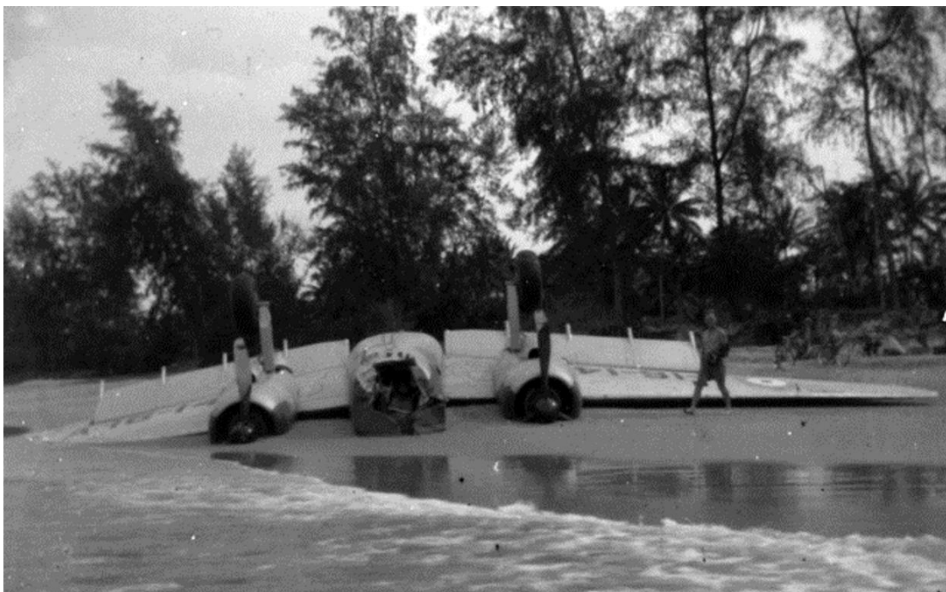
Caption: A16-14 after its accident 1028GMT hrs 23/07/41 when crash landed gear down on beach and flipped, 75 kms on the beach, north of Kuatan, Malaya.
