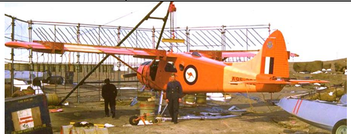
A95-202 with International Orange (FS12197) dayglo band around the rear fuselage and bands across the mainplanes – the image at right shows severe fading of the dayglo (added at Mawson during 1958).
