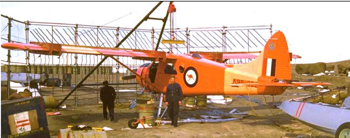
A95-202 with floats and undercarriage removed c1958/59 – the dayglo has severely faded, which may be as it was added in the harsh Antarctic conditions, and outside the temperature specified for applying this high-visibility finish.
