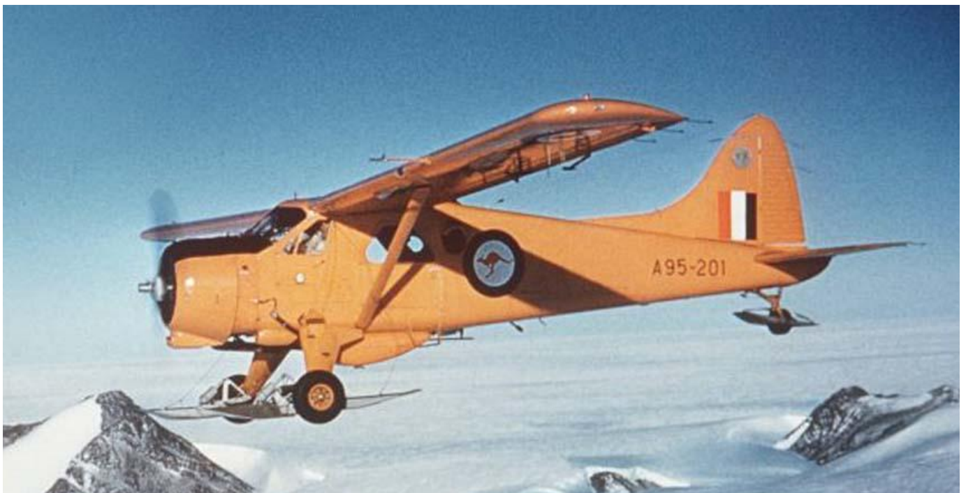
A95-201 in 1959 with the normal Mawson base ski and wheels undercarriage configuration
