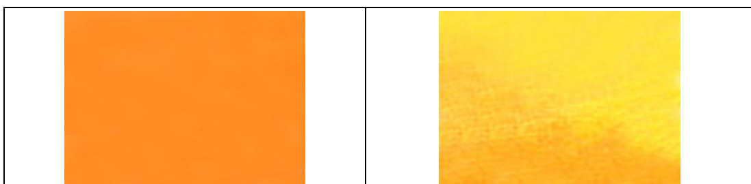
Weathering dayglo – fresh application to A81-3 1965; already A81-4 faded after a year in 1963
