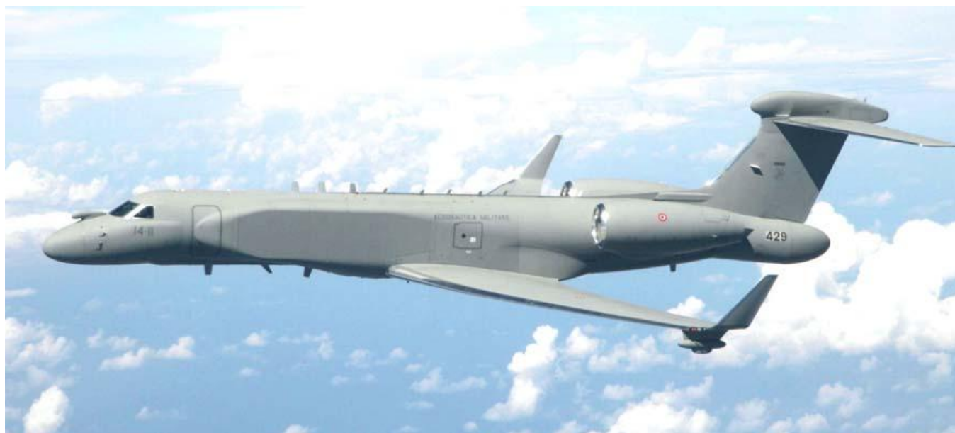
Italian MC-55 (msn 5429) delivered in 2016 with an Israeli conformal antenna – not fitted to the RAAF MC-55A
