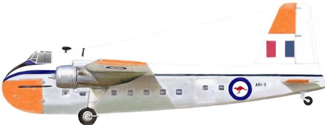
Roundel sizes, diameter inches (cm): fuselage 48" (121.9cm), mainplanes 72" (182.88cm) Fin flash: 36" high, 60" wide (20" each colour)
